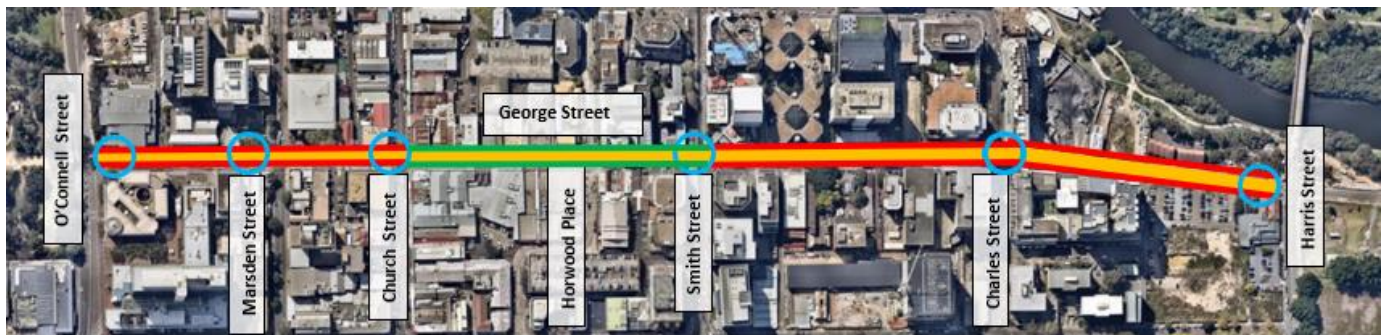
Two-way traffic change Works to lay new asphalt Traffic signal upgrade New line marking
